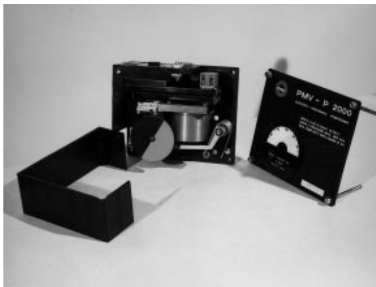
The PMV Positioner with the cover (33) and the side frame (3) dismounted.
